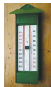
d. Maximum - minimum thermometer
