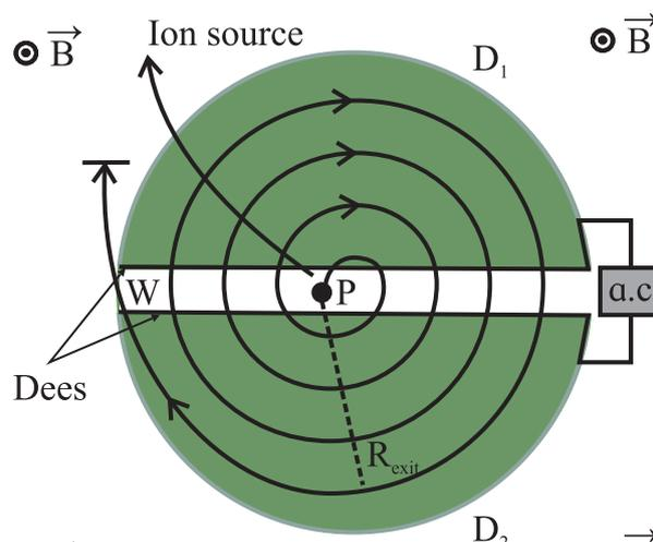
**Fig 10.6: Schematic diagram of a Cyclotron with the two Ds. A uniform magnetic field  $\vec{B}$  is perpendicular to the plane of the paper, coming out. The ions are injected into the D at point P. An alternating voltage is supplied to the Ds. The entire assembly is placed in a vacuum chamber.**
