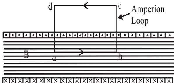
**Fig. 10.25: Ampere's law applied to a part of a long ideal solenoid: The dots (.) show that the current is coming out of the plane of the paper and the crosses (x) show that the current is going into the plane of the paper, both in the coil of square cross section wire.**
