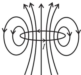
Fig. 10.20: Magnetic field lines for a current loop.
