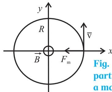
**Fig. 10.5: Charged particle moving in a magnetic field.**
