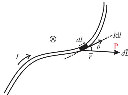
**Figure 10.15: A current carrying wire of arbitrary shape, carrying a current  $I$ . The current in the differential length element  $dl$  produces differential magnetic field  $d\vec{B}$  at a point P at a distance  $\vec{r}$  from the element  $dl$ . The  $\otimes$  indicates that  $d\vec{B}$  is directed into the plane of the paper.**
